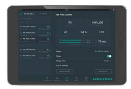
The software makes optimising the aerial alignment respectively determining the location of the repeater a breeze and also serves as a useful tool during set up. The XIRIUM PRO app facilitates the setting of all function parameters (e.g. output power, delay time, etc.) and the monitoring (e.g. signal strength, battery power, etc.). Future functional expansion or performance optimisation of the wireless devices can easily be accomplished via the firmware update function.
