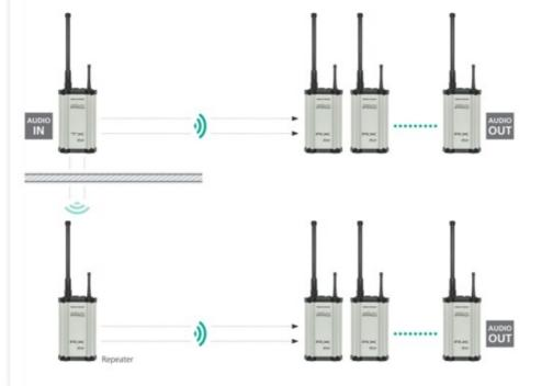
The RX can either be used as a receiver or, by changing the output module to a repeater module, as a repeater. In repeater mode the RX forwards the audio signal received from the TX without any changes, which in turn can now be received by an unlimited number of RX receivers set to reception mode. The repeater represents the perfect addition to the system: it doubles the range of the system and helps to overcome walls, corners or other obstacles.
