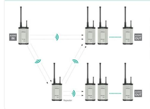
Beside enhancing the range or overcoming obstacles, the RX-repeater offers another feature: since the repeater duplicates and transmits the signals received from the TX, it becomes a second redundant audio source for every other RX. In other words, an RX located within the reception area of an TX and a repeater, can now choose one of two identical signals and automatically selects the one with the better signal quality.
