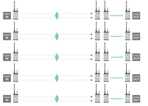
The system may be expanded to ten sound channels for the transmission of several, discrete audio signals. For this purpose five TX transmitters may be operated in parallell. This set up allows the use of an unlimited number of RX receivers.
