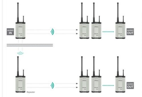
The RX can either be used as a receiver or, by changing the output module to a repeater module, as a repeater. In repeater mode the RX forwards the audio signal received from the TX without any changes, which in turn can now be received by an unlimited number of RX receivers set to reception mode. The repeater represents the perfect addition to the system: it doubles the range of the system and helps to overcome walls, corners or other obstacles.
