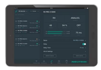
The software makes optimising the aerial alignment respectively determining the location of the repeater a breeze and also serves as a useful tool during set up. The XIRIUM PRO app facilitates the setting of all function parameters (e.g. output power, delay time, etc.) and the monitoring (e.g. signal strength, battery power, etc.). Future functional expansion or performance optimisation of the wireless devices can easily be accomplished via the firmware update function.
