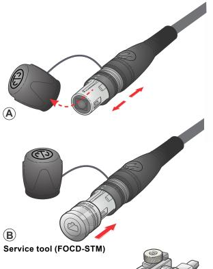
1. Disconnect both cable ends for safety reasons. Invisible laser radiation may be emitted from disconnected fibers or connectors. Do not stare into beams or view directly with optical instruments.
