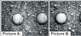
During inspection procedure, make sure that each ferrule is completely free of dust. As a reference the ferrule has to look as illustrated on Picture B.
