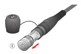
**9.** After the cleaning procedure unlock the NEUTRIK inspection tool (I).
