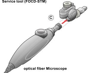
3. Prepare the optical fiber video probe with the correlate singlemode or multimode tip (C). Under the following QR-code you can find a list with appropriate video probs and tips.
