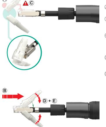
In the case of using shielded cable crimp shield to connector.
