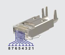
Consider the cable end termination either according to the TIA 568A or T568B standard.
