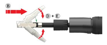
Position the chuck onto the RJ45.
