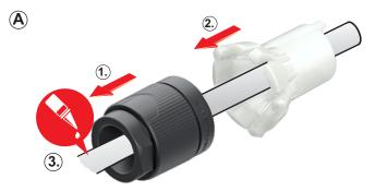
Place the bushing (1) and chuck (2) over the cable.
