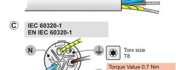
Slide the cable into the contacts and clamp with the screw with Torx size T8.
