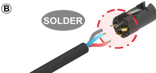
**B** Insert wires into the terminals and solder them.
