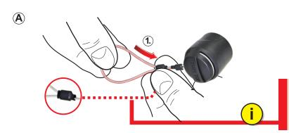
Open the loop 1 of the NEUTRIK sealing cap as shown in the figure A.
