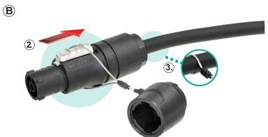
Slide the open loop 2 over the connector and position it at the junction of the cable 3 and the connector.
