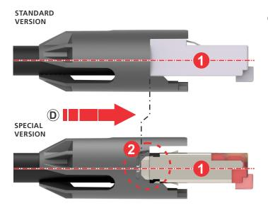
(D) Position the RJ45 in the chuck.
