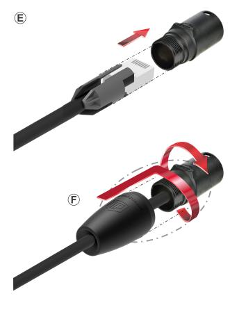
**E** Position the unit (RJ45 and chuck) into the housing.
