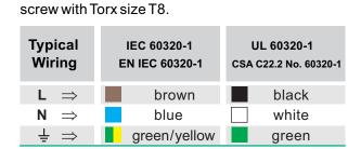
Slide the cable into the contacts and clamp with the
