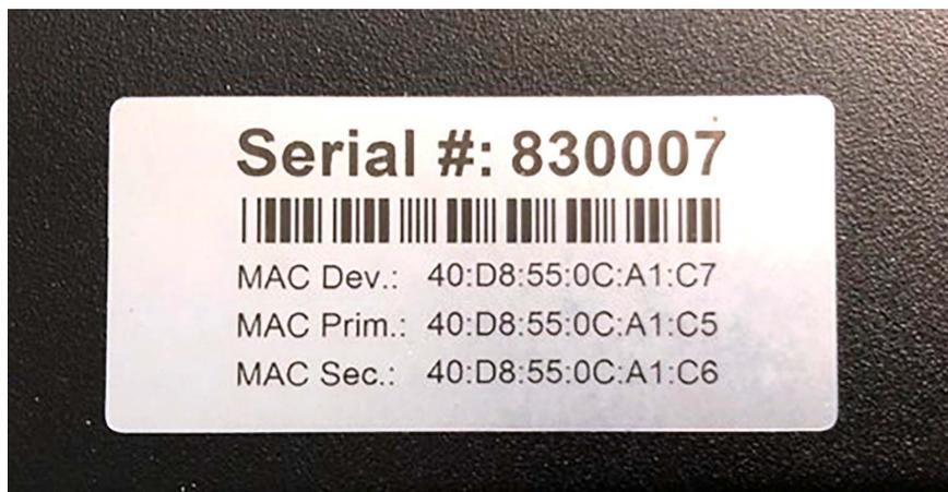
figure 1: MAC addresses on serial number label
