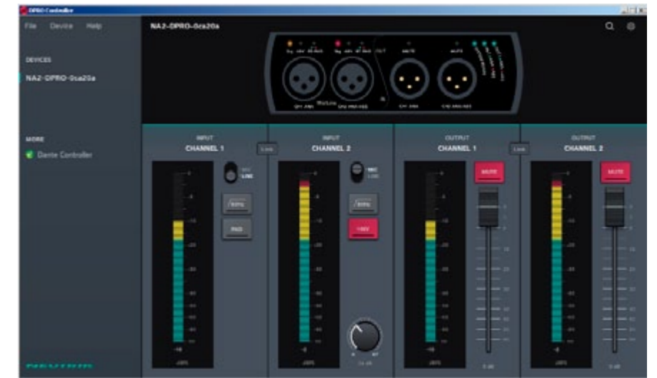
DPRO Controller for setting the NA2-IO-DPRO. For the inputs and outputs, fine resolution level indicators are included that light up yellow from -18 dBfs and red from -3 dBfs onwards
