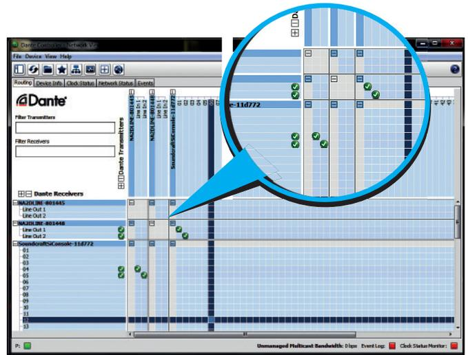
The "Dante™ Controller" software is used only to set up the audio connection (routing) between devices and to configure the subscribing devices. The devices are controlled in the DPRO Controller App.
