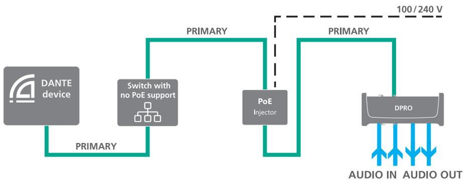
For power and data redundancy, use 2x passive PoE injectors. Because they do not use the discovery process, switching between primary and secondary will not result in a short loss of audio. More information about PoE please find in section "7.2 PoE (Power over Ethernet)" on page 41.
