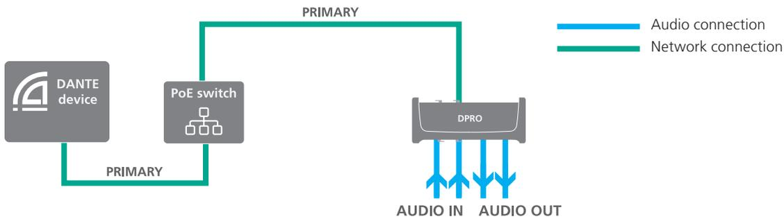
**i** The DPRO Adapter forwards information to the PoE switch indicating that it is a "Class 2" device to ensure the correct power supply.
