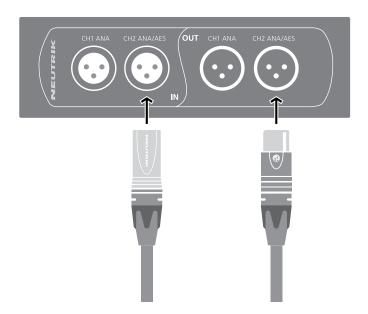
If there is a physical XLR connection on channel 2 only (valid for input & output), the device is operating in AES mode. No audio parameters can be adjusted in DPRO Controller software.
