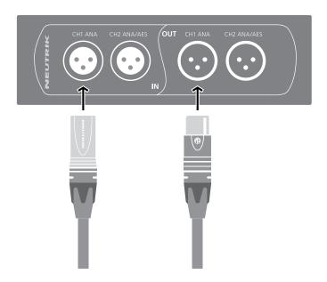
If there is a physical XLR connection to channel 1 only (valid for input & output), the device is operating in analog mode.
