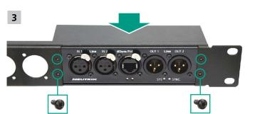
▶ Remove the 4 screws on the front of the device.
