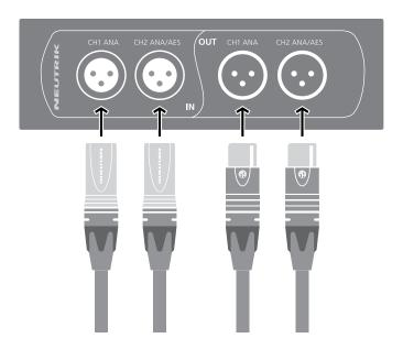
If there is a physical XLR connection to channel 1 & 2 (valid for input & output) the device is operating in analog mode.
