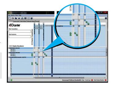
The "Dante™ Controller" software is used only to set up the audio connection (routing) between devices and to configure the subscribing devices.
