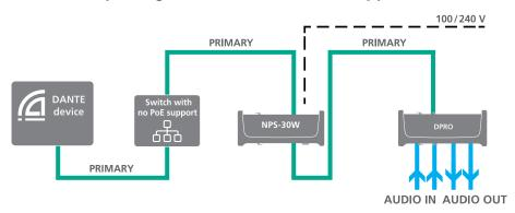
For power and data redundancy, use 2x passive PoE injectors. Because they do not use the discovery process, switching between primary and secondary will not result in a short loss of audio. More information about PoE please find in section "7.2 PoE (Power over Ethernet)" on page 48.
