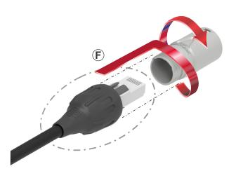
F Slide the unit (insert and boot) into the housing and tighten the bushing.
