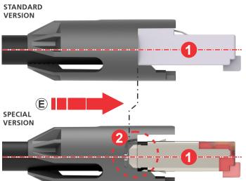
(E) Position the RJ45 in the chuck.
