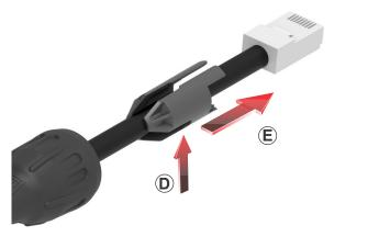
Put the chuck onto the cable.Align the opening with the contact side.
