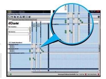
The "Dante™ Controller" software is solely used to set up the audio connection (routing) between devices and to configure the involved devices.
