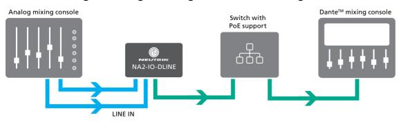
Here, the Dante<sup>™</sup> adapter is used to integrate up to 2 analog LINE signals into a Dante<sup>™</sup> system.
