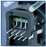
Vertical PCB with lightpipes
