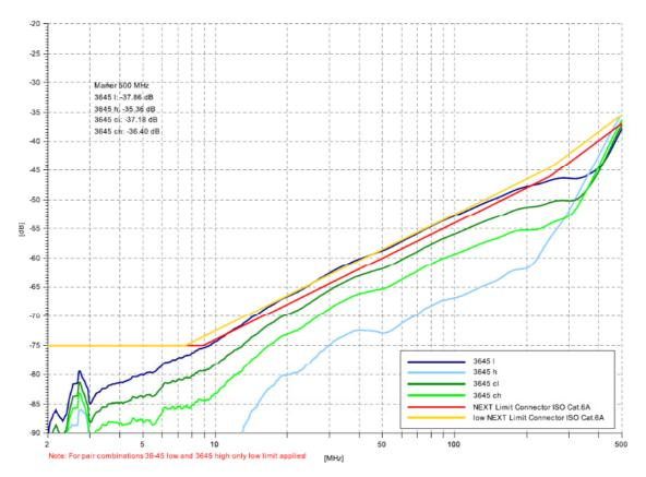
For pair combinations 3645 high and 3645 low, only the low NEXT limits apply. The combination 3645 low meets the standard values within the accuracy of the test equipment.
