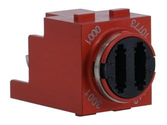
Benefiting from the expanded beam technology and the precision optical alignment the system creates high immunity against dust, mud, liquids and other contaminations. The FIBERFOX foxBRID module converts a standardized LC Patch cable into an expanded beam solution. It acts as a "feed-through" and fits into industrial standard shells.
