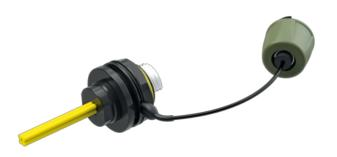
Benefiting from the expanded beam technology and the precision optical alignment the system creates high immunity against dust, mud, liquids and other contaminations. The FIBERFOX EBC25 4CH chassis connector converts a standardized LC patch cable into an expanded beam solution. It acts as a "feed-through" and has a jam nut design.
