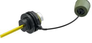
Benefiting from the expanded beam technology and the precision optical alignment the system creates high immunity against dust, mud, liquids and other contaminations. The FIBERFOX EBC25 2CH fixed patch cable connector converts a standardized LC patch cable into an expanded beam solution. It acts as a "feed-through" and has a jam-nut design
