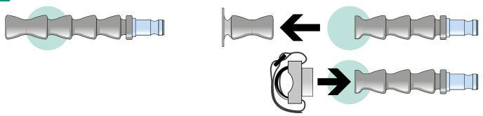
Press the provided adapter module onto the mounting arm and attach it to the antenna with the fastener.
