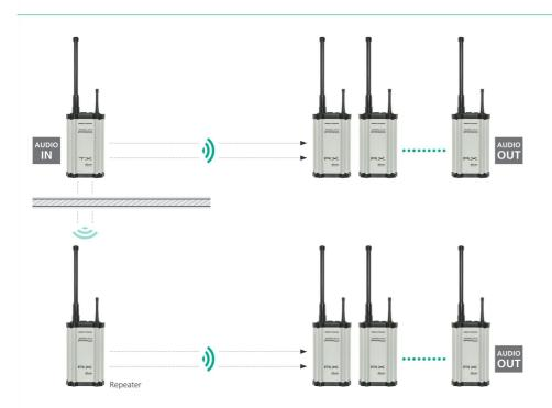
The RX can either be used as a receiver or, by changing the output module to a repeater module, as a repeater. In repeater mode the RX forwards the audio signal received from the TX without any changes, which in turn can now be received by an unlimited number of RX receivers set to reception mode. The repeater represents the perfect addition to the system: it doubles the range of the system and helps to overcome walls, corners or other obstacles.
