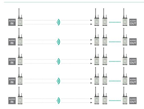
The system may be expanded to ten sound channels for the transmission of several, discrete audio signals. For this purpose five TX transmitters may be operated in parallell. This set up allows the use of an unlimited number of RX receivers.
