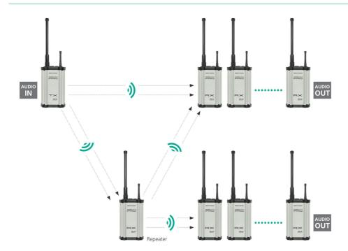
Beside enhancing the range or overcoming obstacles, the RX-repeater offers another feature: since the repeater duplicates and transmits the signals received from the TX, it becomes a second redundant audio source for every other RX. In other words, an RX located within the reception area of an TX and a repeater, can now choose one of two identical signals and automatically selects the one with the better signal quality.
